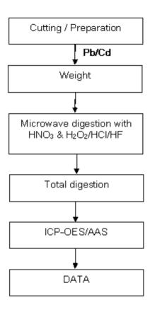
The samples were dissolved totally by pre-conditioning method according to above flow chart.
